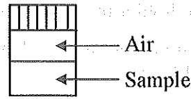
Illustration 3-5. Setting sample in vial bottle
